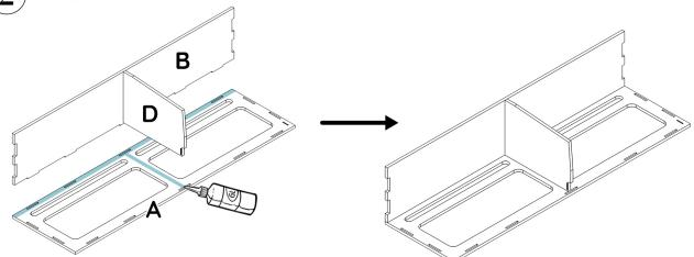
${f 2}$  Apply glue to the notches and joints then assemble part  ${f c}$  with the rest of the furniture.
