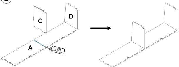
(3) Apply glue to the notches and joints then assemble part **B** with the rest of the furniture.
