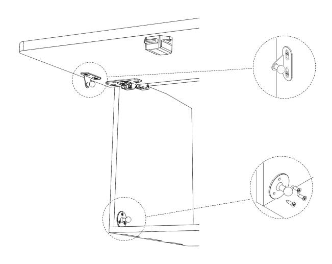
(3.2) Insert the bases into the struts on each side of the furniture.
