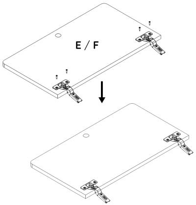
(2.2) Fix the hinge bases to the cabinet by screwing the 15mm screws into the pilot holes as shown below.
