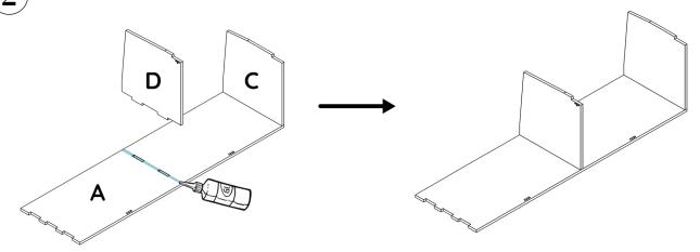
(3) Apply glue to the notches and joints then assemble part **B** with the rest of the furniture.
