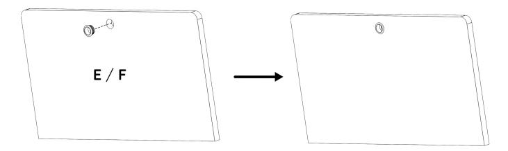
(1.2) Screw the button onto the push lock.
