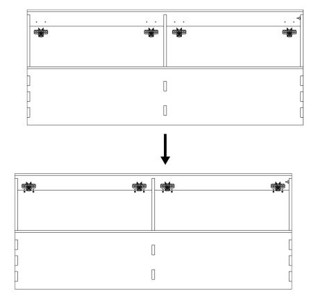
(2.3) Assemble the door hinges onto the bases fixed to the furniture as shown below.
