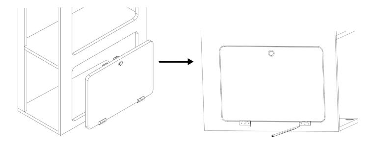
Align one hinge with the front of the cabinet and fold it down over the front of the cabinet to match the previously marked hole. Then screw in a 12mm screw (hole in the middle of the hinge). Unscrew the hinge and repeat this process to mark the hole for the second hinge, then unscrew the hinge.
