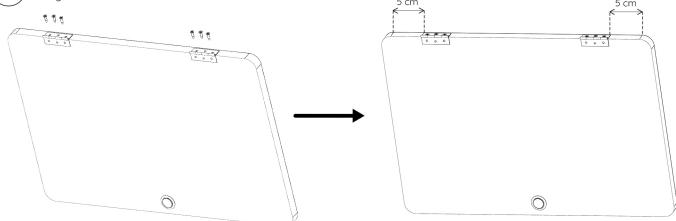
Position the door (**door G** in this example) in its frame and center it, then fold the hinge onto the front of the furniture and make a slight mark using a pencil or tape.
