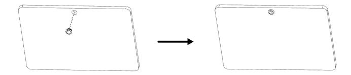
Screw the button onto the push lock..
