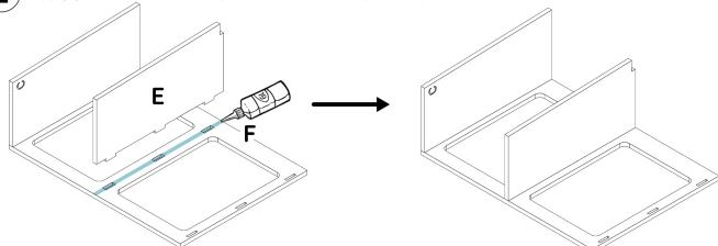
$(\,3\,)\,$  Apply glue to the notches and junction and assemble part **D** onto part **F**.
