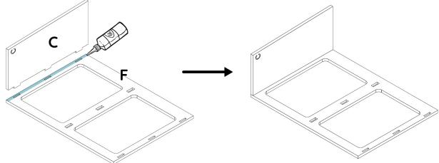
(2) Apply glue to the notches and junction and assemble part **E** to part **F**.
