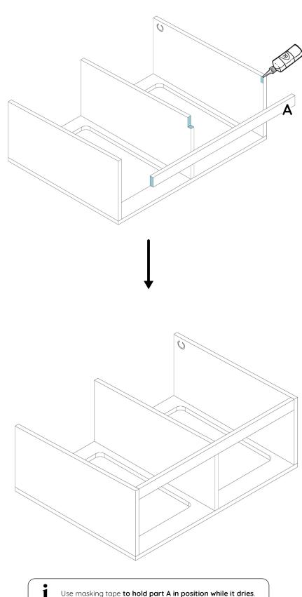
Use masking tape to hold part A in position while it dries.
