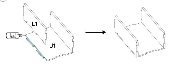
ig(1.3ig) Apply glue to the notches and joints and assemble part M1 with the J1/K1/L1 assembly.
