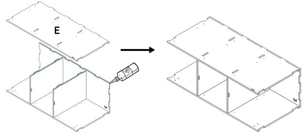
(5) Apply glue to the notches and joints and assemble part **F** with the rest of the furniture.
