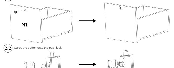
(2.3) Screw the push lock with two 12 mm screws onto door **N1**. Make sure it is aligned with the top of the front panel.
