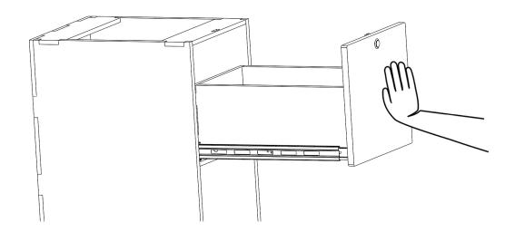
To **adjust the drawer height**, loosen the drawer slide mounting screws, move the drawer up or down, and retighten the 15 mm screws.
