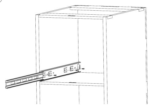
3.3 Screw the slides into the pilot holes in the drawer using the 15 mm screws (3 per slide) on parts K1 and L1.
