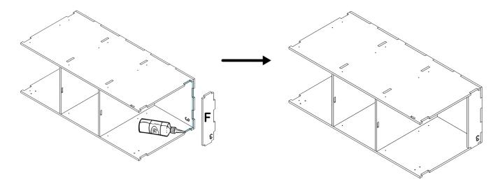
$(\mathbf{6})$  Apply glue to the notches and joints and assemble part **G** with the rest of the furniture.
