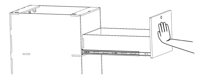
To adjust the drawer height, loosen the drawer slide mounting screws, move the drawer up or down, and retighten the 15 mm screws.
