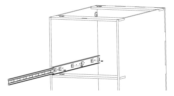
(3.3) Screw the slides into the pilot holes in the drawer using the 15 mm screws (3 per slide) on parts **J** and **K**.
