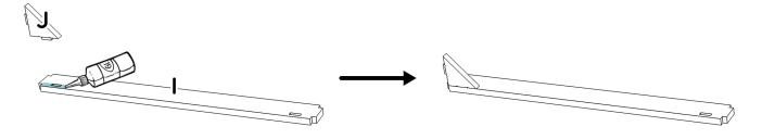
igg(2igg) Apply glue to the notches and junctions then assemble part **B** with the **I/J** assembly.
