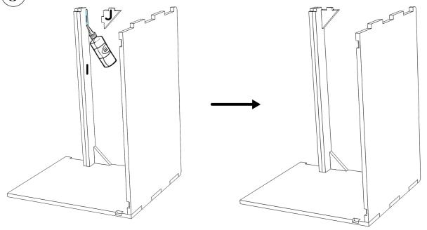
Apply glue to the notches and joints then assemble part **A** with the rest of the furniture.
