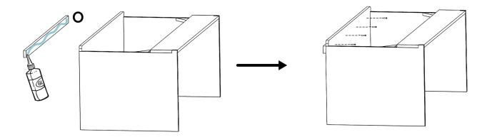
Apply glue to the joints and then assemble part **P** with the rest of the furniture, then screw it from the inside of the furniture with four thin 25 mm screws. **Be careful to align this part well.**
