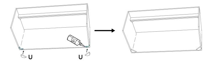
Apply glue to the joints, then assemble part **O** with the rest of the furniture, then screw it from the inside with four thin 25 mm screws. **Be careful to align this part well**.
