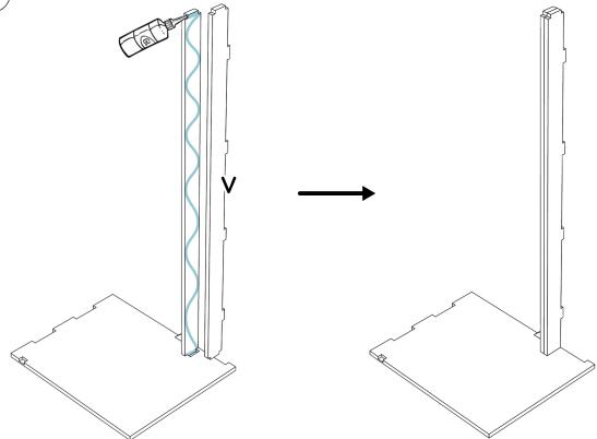
$m{4}$  Apply glue to the notches and joints then assemble part **S** with the rest of the furniture.
