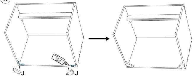
Apply glue to the joints, then assemble part **G** with the rest of the furniture, then screw it from the inside with four thin 25 mm screws. **Be careful to align this part well.**
