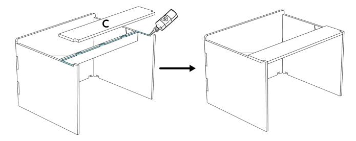
Apply glue to the notches and joints then assemble two **J** angles as below.
