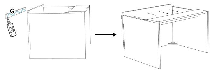
Apply glue to the joints and then assemble part  $\mathbf{F}$  with the rest of the furniture, then screw it from the inside of the furniture with four thin 25 mm screws. **Be careful to align this part well.**
