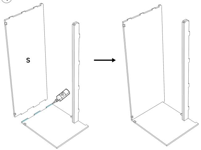
$\overbrace{\mathbf{5}}$  Apply glue to the notches and joints then assemble a **U** angle with the **T** piece.
