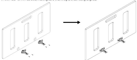
(2) Screw the crosshead bases into the pilot holes with four 15mm screws.
