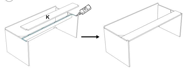
iggsep Apply glue to the notches and joints then assemble two  $oldsymbol{U}$  angles as shown below.
