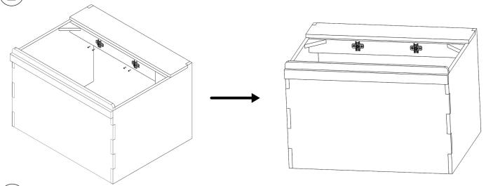
(3) Assemble the top hinges onto the bases fixed to the furniture as shown below.
