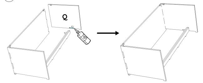
(7) Apply glue to the notches and joints then assemble part **K** with the rest of the furniture.
