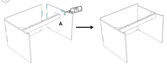
(7) Apply glue to the notches and joints then assemble part **C** with the rest of the furniture.
