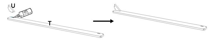
(2) Apply glue to the notches and joints then assemble the **R** part with the **U/T** assembly.
