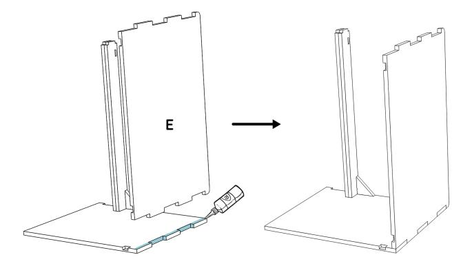
(f 5) Apply glue to the notches and joints then assemble a **J** angle with part **I**.
