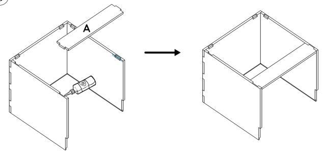
$igg( oldsymbol{9} igg)$  Apply glue to the notches and joints and assemble the two  $oldsymbol{H}$  angles with the rest of the furniture.
