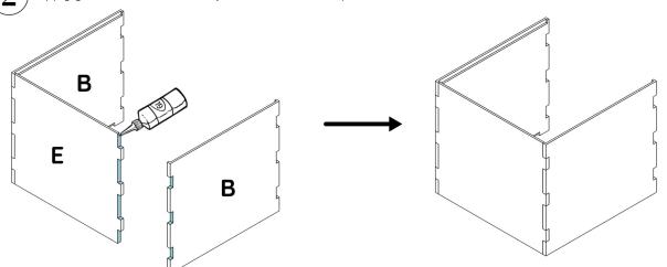
(3) Apply glue to the notches and joints then assemble part **E** with the rest of the furniture.
