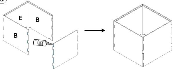
$oxed{4}$  Apply glue to the notches and joints and assemble the four **H** angles with the rest of the furniture.
