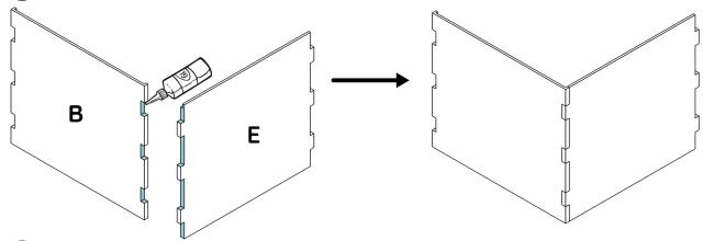
$oldsymbol{\widehat{}}$  Apply glue to the notches and joints then assemble parts **B** and **E**.
