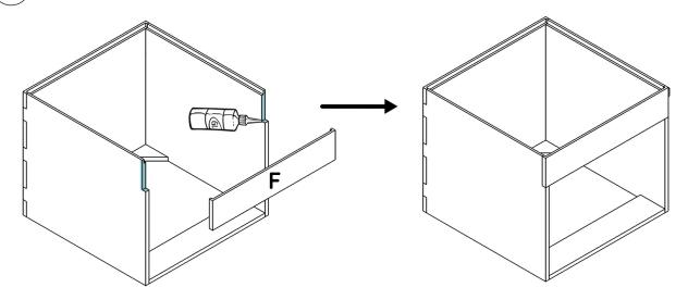
Apply glue and assemble part  ${\bf I}$  with the rest of the furniture, then screw part  ${\bf I}$  from the inside of the furniture using 3 thin 25 mm screws.
