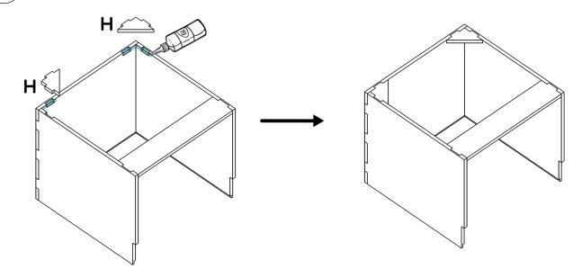
$\widehat{10}$  Apply glue to the notches and joints and assemble part **F** with the rest of the furniture.
